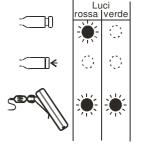
If the point is not pressed, the red light should turn on.
