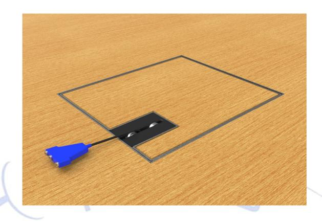
The Floor Box is a device for the placement of a cable reel used in the sport of fencing, built into the sport-floor system. The Floor Box can be installed on a sport-floor glued onto concrete flooring, as well as a swinging floor system built onto concrete flooring. The design of the Floor Box fits the sport-floor layers used on the site of installation, thus it may be vinyl sport-floor as well as sport hardwood tiles.
