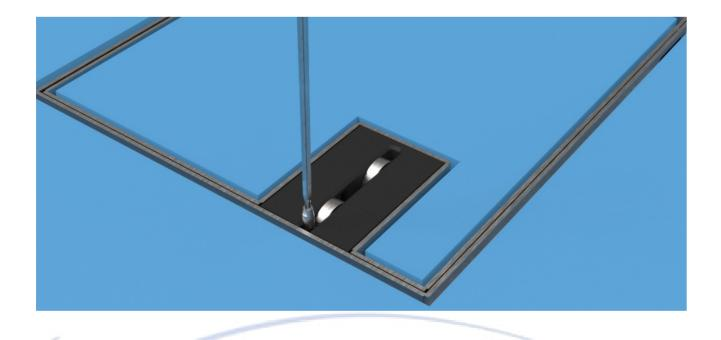
To open it, push the point of the weapon vertically down, into the gap between the guiding roller and the frame. After a slight press the lock opens and the cover moves a little from the surface of the floor. Open the cover by cautiously grabbing the gap.
